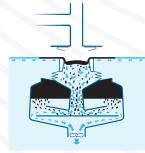
Deflection disks force the pollution and the water to the periphery. As the flow velocity drops, the pollution floats upwards while the water flows down through the outlet.
