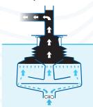
With the water acting as a piston, the pollution is discharged at the rate of up to 8,000 liters per hour into an external container. Recovered oil has a water content of less than 0.5%.
