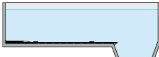
Z 2003/4 Version with horizontal hydraulic cylinder, available with pulling or pushing scraper.
