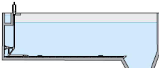
Z 2001/2 Hydraulically operated pushing scraper with central cylinder frame, mounted on a concrete base.
