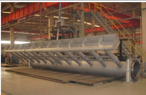
Factory Preassembly & Dry-run Test
