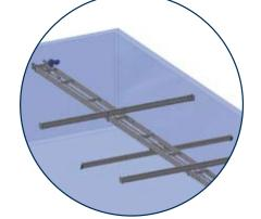
> Only the scraper blade comes into contact with the surface of the water. When it reaches the end of its travel and has deposited the scum, the blade is angled up again for the return movement. Several scraper blades can be used in the same tank.
