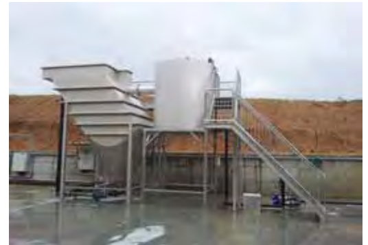
MODELL LS IS A SEPARATOR WITH SLUDGE THICKENING BOTTOM HOPPER
