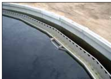
KD 16.08 Scum outlet, fitted directly to KD 16.18 stainless steel channel, where the side facing the centre part acts as scum board. Can also be fitted to KD 16.17 scum board.
