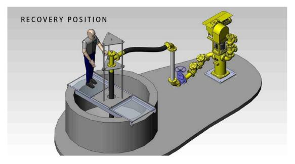
The cost of the EMS dredging pump is much more than the cost of an airlift or centrifugal pump but weighed against this is the saving of not having to buy and maintain a mechanised propeller arrangement.
