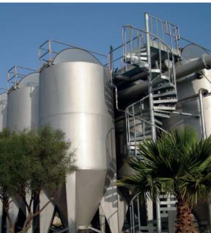
A typical installation of DynaSand DS5000 AD HD. The filters have lids and do not need covering.
